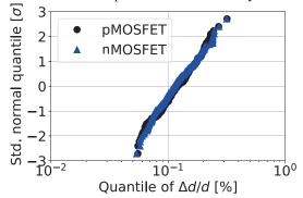
Fig. 4: QQ plot of RTN induced  $\Delta d/d$  for pMOSFET and nMOSFET dominant ROs.
