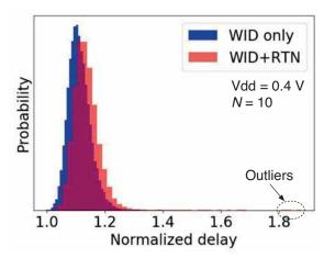
Fig. 10: Histograms of simulated delay. Outliers appear in the case of considering RTN induced  $\Delta V_{\rm T}$  variation.
