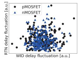
Fig. 6: Correlation between WID delay variation and RTN induced delay fluctuation. No correlation is observed.
