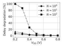
Fig. 11: Increase of worst-case delay due to RTN against that without RTN.
