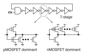
Fig. 1: Ring oscillator structure to characterize pMOSFET and nMOSET RTN. Large skewed inverter cells are used. Different P/N ratio is utilized to decouple nMOSFET and pMOSFET RTN.
