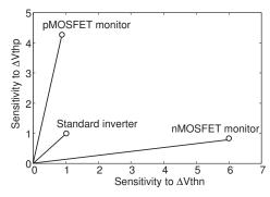
Fig. 3. Sensitivity vectors of proposed process monitors and RO with standard inverter cell. Vectors of the process monitors are near orthogonal, thus suitable for process corner detection.
