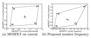
Fig. 4. MOSFET on currents (a) and monitor frequencies (b) simulated at the process corners. Monitor frequencies are distributed in the process space.
