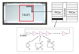
Fig. 5. Test chip structure. ROs consisting of the proposed inverter structure and the standard inverter structure are implemented.
