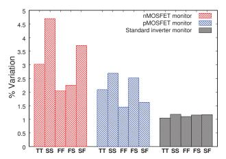
Fig. 7. WID variation observed in nMOSFET monitor, pMOSFET monitor and standard inverter ROs at the corner chips.
