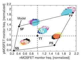
Fig. 6. Measured monitor frequencies from 5 chips per corner. Each chip contains 294 instances of each monitor.
