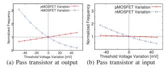
Fig. 2. Sensitivity to MOSFET threshold voltage variation. Structure of (b) is sensitive to particular MOSFET variation thus suitable for parameter extraction.
