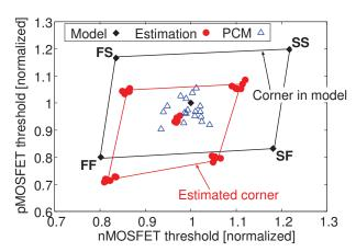
Fig. 8. Comparison between threshold voltage corners defined in transistor model and measured by monitor circuits.
