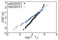
Fig. 8: CDF of WID leakage variation for nMOSFET and pMOSFET. The distribution fits log-normal distribution.
