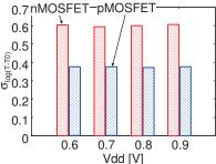
Fig. 9: Measured leakage variation at several supply voltage.
