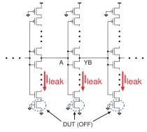
Fig. 5: Homogeneous structure to monitor average nMOSFET leakage current.
