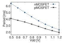
Fig. 10: Measured oscillation period due to N MOSFETs' leakage current at different supply voltages.
