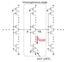
Fig. 4: Inhomogeneous structure to monitor single nMOFSET leakage current.
