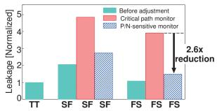
Fig. 9. Leakage measurement for "TT", "SF" and "FS" chips when (a) both MOSFETs are biased uniformly and (b) proposed scheme is applied.
