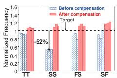
Fig. 8. Frequencies of ROs consisting of various kinds of gates, INV, NAND and NOR frequencies are plotted for each corner from the left.
