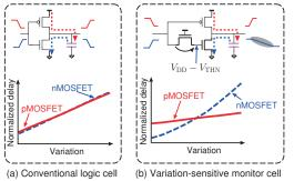
Fig. 2. Sensitivity of the proposed monitor cell compared to conventional logic cells. The proposed monitor cell is sensitive to a particular type of MOSFET variation only.
