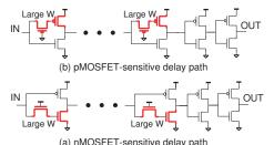
Fig. 4. Proposed variation-sensitive monitor circuit structure. Pass-gate at input makes the delay highly sensitive to MOSFET variation.
