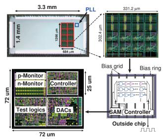
Fig. 5. Chip photograph and layout of the self-adjustment scheme. ROs of several logic gates are implemented to evaluate critical path delays.
