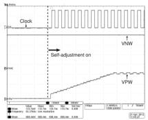
Fig. 6. Measured transient response of the self-adjusting module when self-adjustment is enabled. System stability and independent control of body bias is confirmed.
