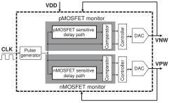
Fig. 3. Schematic of built-in self-adjustment scheme. P/N variations are detected comparing the clock with the delays of monitor paths. System supply and clock is used to generate body voltages.
