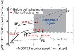
Fig. 7. Output performances of pMOSFET-sensitive and nMOSFET-sensitive ROs. Performances are measured before and after self-adjustment. Generated body biases for each corner are shown in closed bracket.
