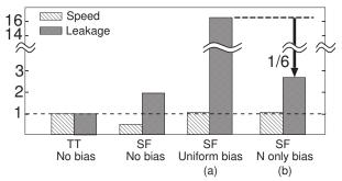
Fig. 1. Circuit speed and leakage for two corners of "TT" and "SF". Forward body bias is applied for "SF" corner to compensate speed based on (a) critical path monitoring (uniform bias) and (b) P/N-sensitive monitoring (N only bias).
