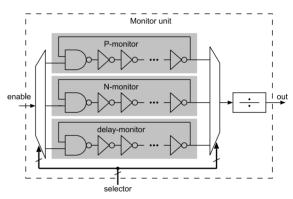
**Fig. 2** One example of monitor unit. The monitor unit consists of three process monitors here to detect process shift and process spread.
