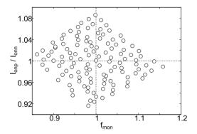
**Fig. 7** Correlation between ON-current ratio of MOSFETs,  $I_{\text{onp}}/I_{\text{onn}}$  and standard inverter based process monitor frequency.
