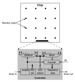
**Fig. 1** One example of on-chip implementation of monitor circuits. Conventional scan-chain based interface is used in this example.
