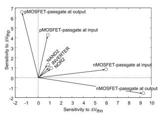
Fig. 5 Sensitivity vectors of pass-gate based process monitors and RO with standard inverter. NAND2 and NOR2 cells.
