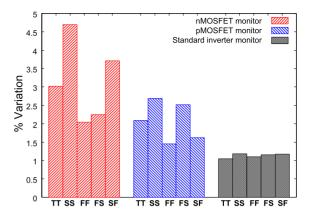
Fig. 11 WID variation observed in nMOSFET monitor, pMOSFET monitor and standard inverter ROs at the corner chips.
