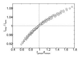
**Fig. 8** Correlation between MOSFET ON-current ratio,  $I_{\rm onp}/I_{\rm onn}$  and monitor frequency ratio  $(f_{\rm pmon}/f_{\rm nmon})$ . High correlation coefficient of 0.98 is found. The p- and n-monitors can detect P/N-ratio with high accuracy.
